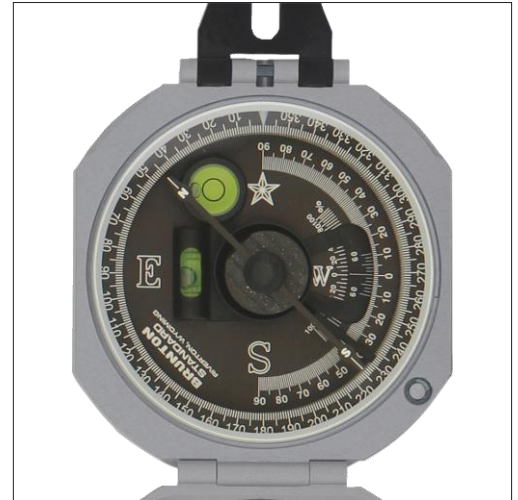
updated needle with NeFeB Disk Magnet improves shock resistance
